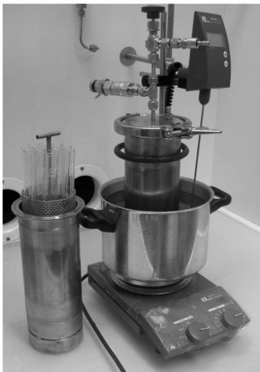
Figure 1. Photograph of the reaction setup; the left-hand side shows an opened reaction autoclave with 14 glass reactors inside, and the right-hand side presents the autoclave as it appears during the reactions.
